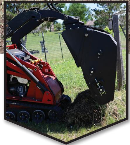
An attachment that pays for itself in a very short amount of time, replacing your hand labor work crew. The Mini Landscape Rake was designed to remove small to medium-sized rock as small as 3/4" along with unwanted roots and debris. The Mini Landscape Rake also breaks up lumpy soil, while grading, leveling, scarifying - preparing the soil in a one-step process. This is the perfect tool for preparing a seedbed, sodding or lawn leveling.
