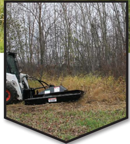
The Rotary Brush Mower / Brush Cutter has been re-engineered for rugged durability, safety, and ease of operation. The 66", 72" and 78" models are built from 1/4" steel making them some of the strongest brush mowers manufactured. This is the most versatile mower on the market today. Use it to cut trees, brush, and unwanted weeds and grass. Its unique automatic Float-n-Tilt™ system allows you to cut evenly on level surfaces, as well as the most rugged terrain.
