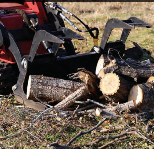
DUAL INDEPENDENT GRAPPLES FOR GRIPPING UNEVEN LOADS
