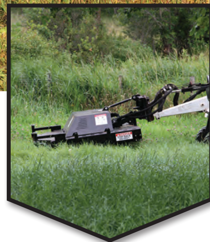
STANDARD RUBBER SHIELDED FRONT GUARD TO PREVENT FLYING DEBRIS
