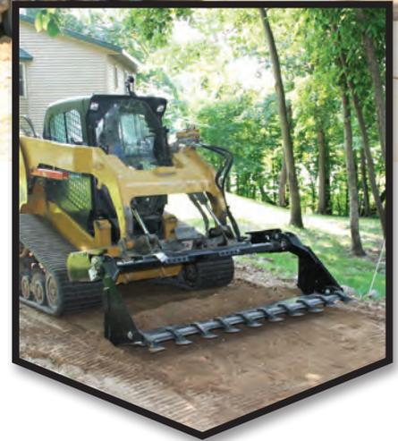
Municipal, landscaping, demolition, and construction sites is where this belongs. This combination bucket does it all: dozing, grappling, leveling, digging, loading, and dumping. Its interlocking serrated grapple edges hold objects securely while its unique design provides digging force.
